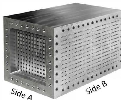
Figure 7: Typical view of a K3-size HER core module (Side A: reactive channels; Side B: heat transfer channels)
