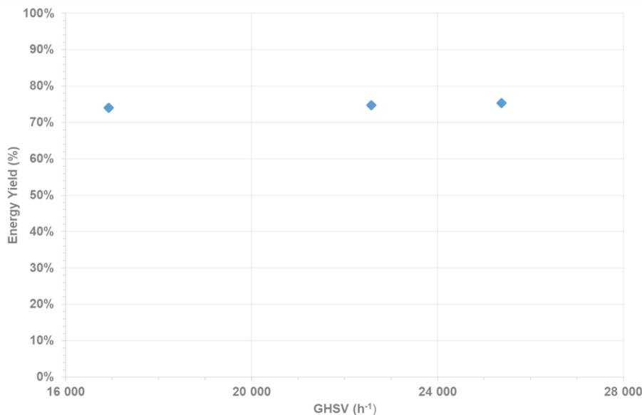
**Figure 14: Energy yield as a function of GHSV, for Operating Temperature = 300°C, Operating Pressure = 5 bar g and H<sub>2</sub>:CO<sub>2</sub> ratio = 4.2:1**
