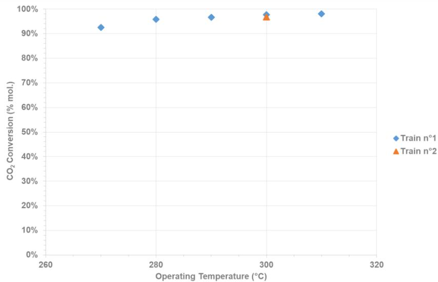
**Figure 11: CO<sub>2</sub> conversion as a function of Operating Temperature, H<sub>2</sub> Inlet Flowrate of 45 Nm<sup>3</sup>/h, Operating Pressure = 5 bar g and H<sub>2</sub>:CO<sub>2</sub> Ratio = 4.2:1**
