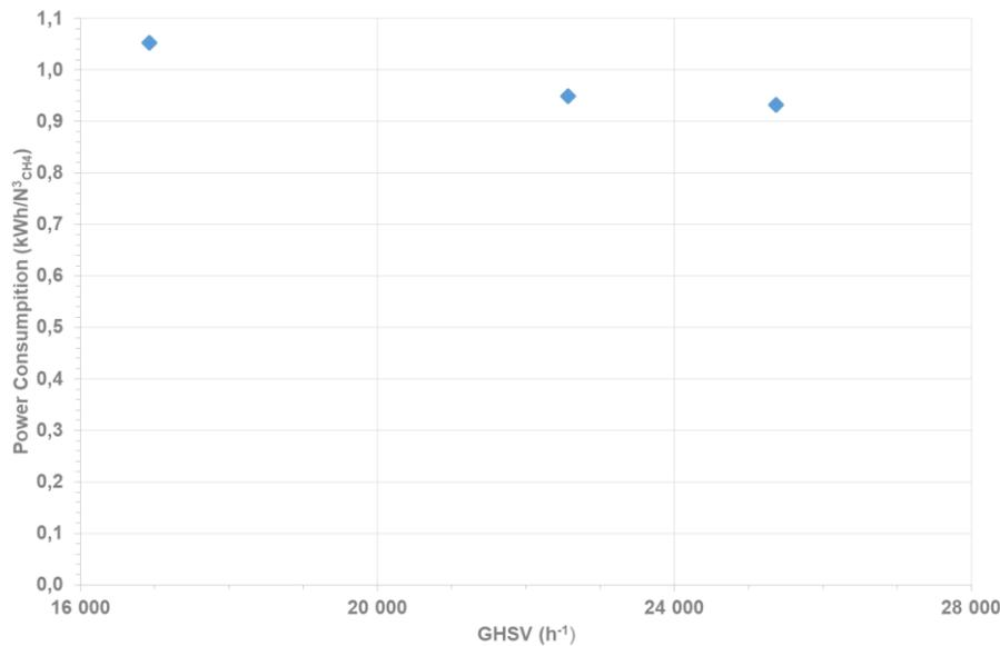
**Figure 13: Power consumption as a function of GHSV, for Operating Temperature = 300°C, Operating Pressure = 5 bar g and H<sub>2</sub>:CO<sub>2</sub> ratio = 4.2:1**
