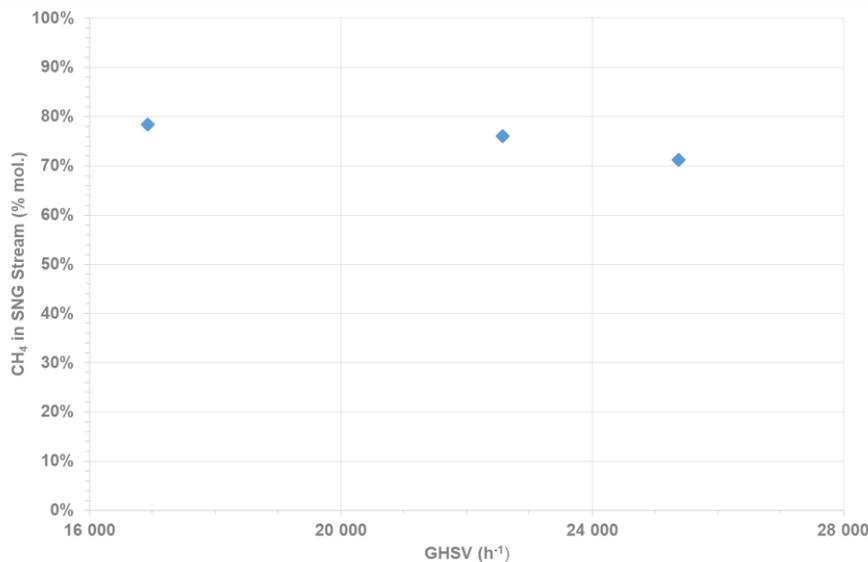
**Figure 12: CH<sub>4</sub> content in the SNG Stream as a function of GHSV, for Operating Temperature = 300°C, Operating Pressure = 5 bar g and H<sub>2</sub>:CO<sub>2</sub> ratio = 4.2:1**
