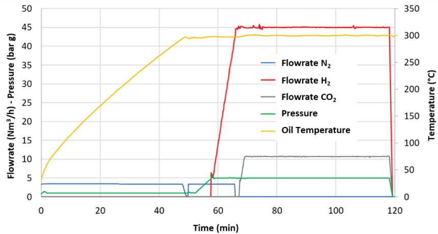
Figure 15: evolution of the main operating parameters after a cold start (train n°1)
