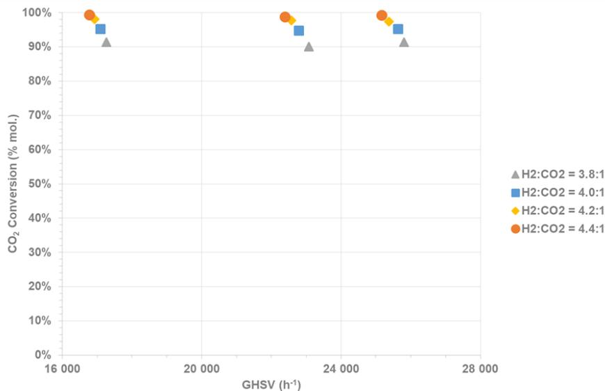
**Figure 10: CO<sub>2</sub> conversion as a function of GHSV for various H<sub>2</sub>:CO<sub>2</sub> ratios, for Operating Pressure = 5 bar g and Operating Temperature = 300°C**
