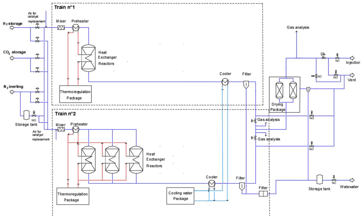
**Figure 4: simplified PFD of the methanation process**
